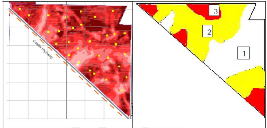
Figure 1. Sea Lake 2011 site maps showing: Left: EM survey map [dark red= highest EC; lighter red= lower EC]. Right: Paddock zones (1= high production zone; 2= lower production zone; 3= lowest production zone)
